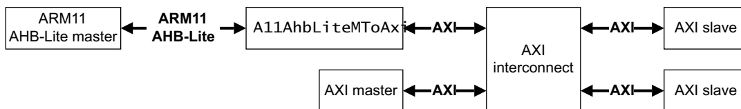
Figure 1-2 ARM11 AHB-Lite master to AXI interconnect example
